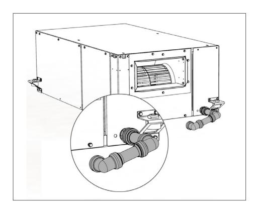
The front drain connection accessory kit includes parts to relocate the condensate drain from the back (discharge) end location, to the front of the unit (supply and return connections) end.
