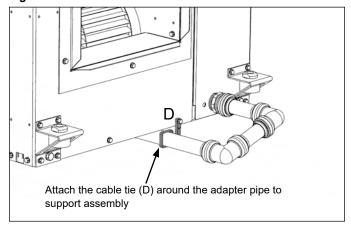
**Note:** To prevent leaks due to sagging, ensure there is no stress or strain from unsupported weight on the connection points of the fittings.
